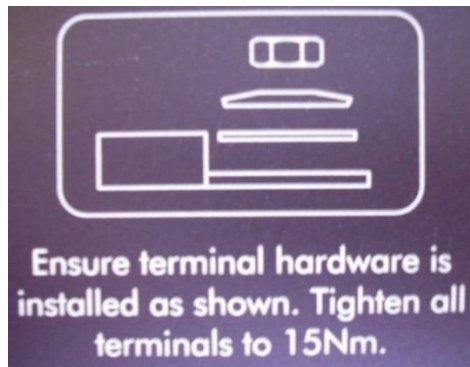
Figure 12 – Power Terminal Hardware Stack Up
