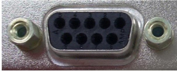
Figure 23: Image of Communication Connector at Cabinet Bulkhead
