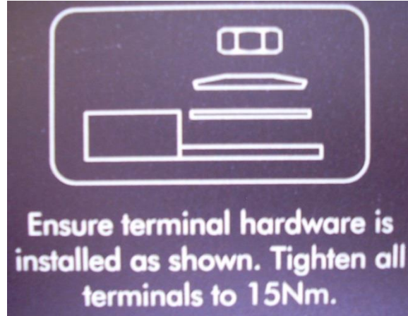
Figure 7: Power Terminal Hardware Stackup
